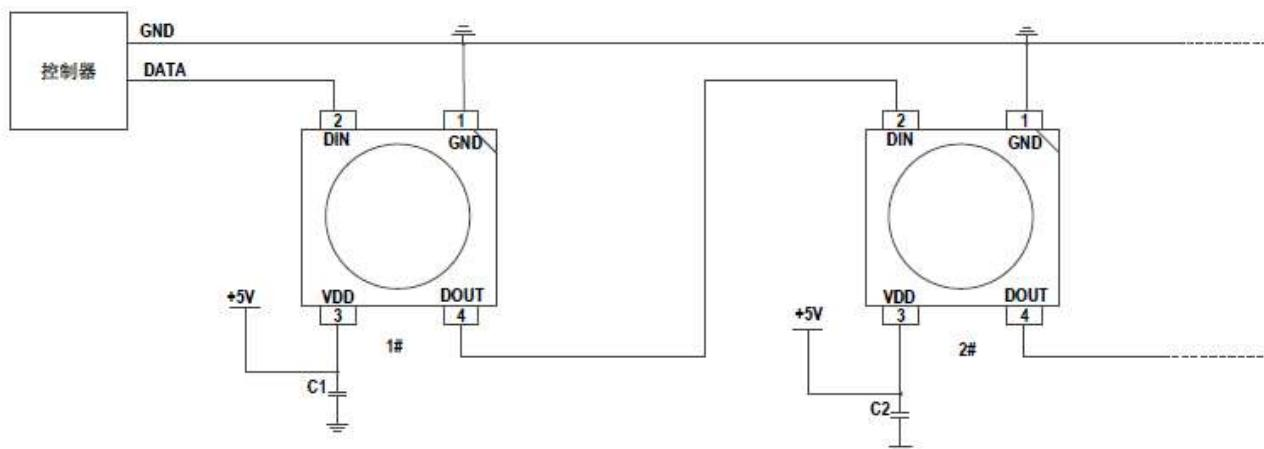
Note: in the above application diagram, C1 and C2 are 100nF / 50V ceramic chip capacitors
